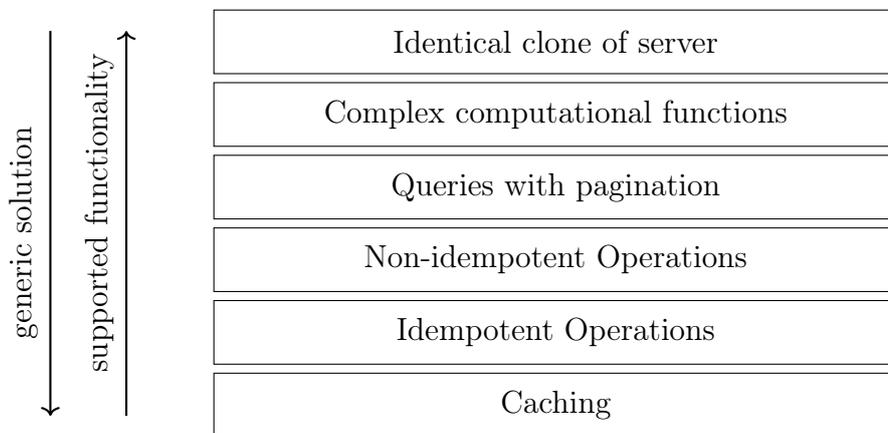
**Figure 2.1:** A six-tier hierarchy for offline support.
