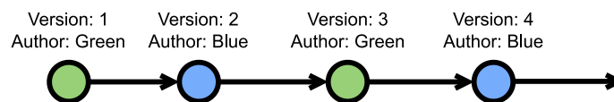
Figure 2.2: Document edited by different authors, document versions are in a global total order
