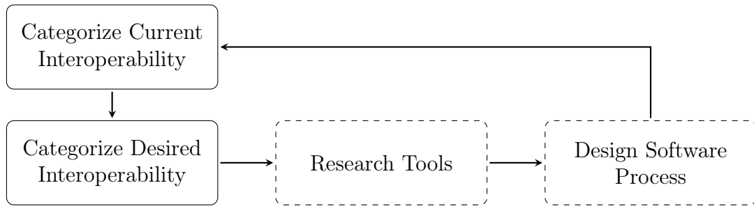
Figure 4.3: Intended usage of the categorization system. The dotted boxes are fully project-specific and therefore not part of this thesis.
