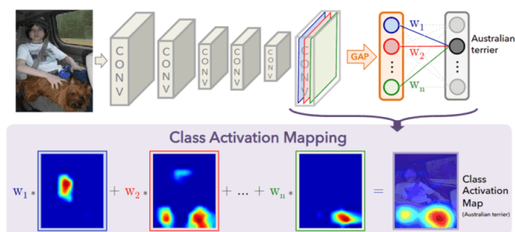
Figure 2.1: Grad-CAM pipeline showing how gradients weight convolutional feature maps to produce a class activation map. Adapted from Selvaraju( Selvaraju et al., 2017b).
