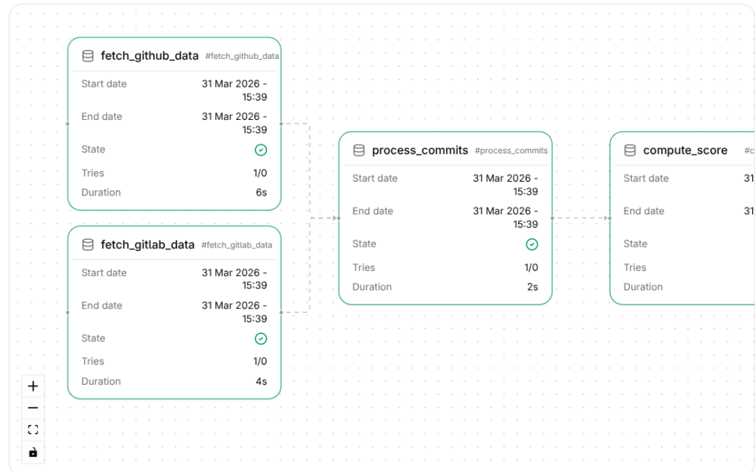
Figure 5.4: Interactive DAG Visualization Embedded in the Workflow Page for Structural Inspection of Task Dependencies
